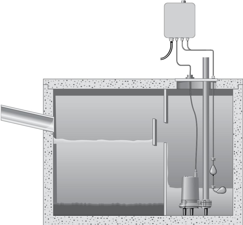
*Typical Three Phase Simplex Installation with float*
